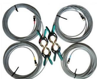
H winding test cable set
