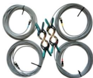
H winding test cable set
